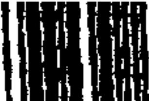
In these cases the bars have joined together in certain places, which makes it difficult for the toolkit to separate the bars and determine their relative sizes.
